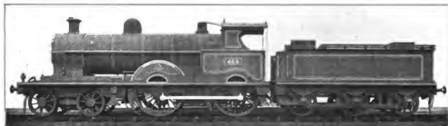
Fig. 5048. Eight-Wheel, Four-Coupled Locomotive. London & North Western. Cylinders 19 in. x 26 in.; Working Steam Pressure 175 lbs. per sq. in.; Total Heating Surface 2,009.7 sq. ft.; Diameter of Drivers 81 in.
